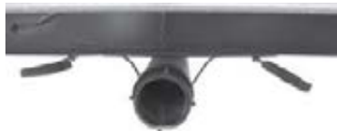
Black/Grey Tank Drain and Valves
