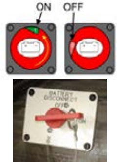
Battery Disconnect Switches
